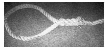
Figure D-018 3-Strand Splice of Poor Quality
