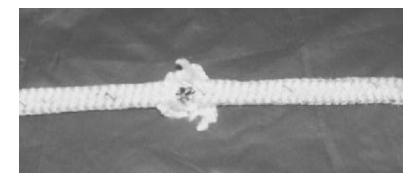
Figure D-012 Cut in Jacket Exposing Core
