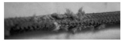
Figure D-009 Localized Jacket Wear
