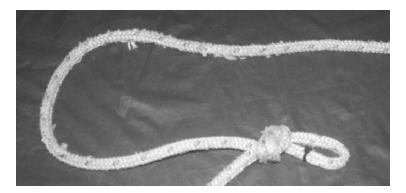
Figure D-022 Knot in Non-Spliceable Rope
