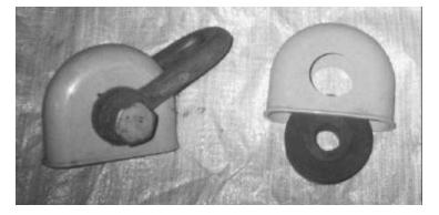
Figure 9 Plastic Thimble for Fiber Rope
