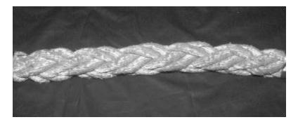
Figure 2 8-Strand Plaited Rope
