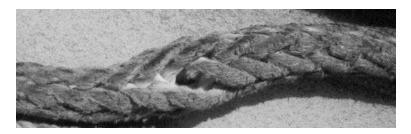
Figure D-003 Inter-Strand Abrasion
