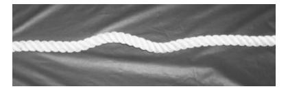
Figure D-024 Corkscrew Due to Twist
