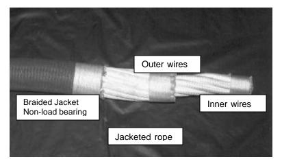
Figure 5 Wire Lay Rope
