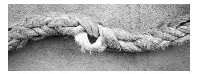
Figure D-013 Pulled Strand in 8 Strand Rope
