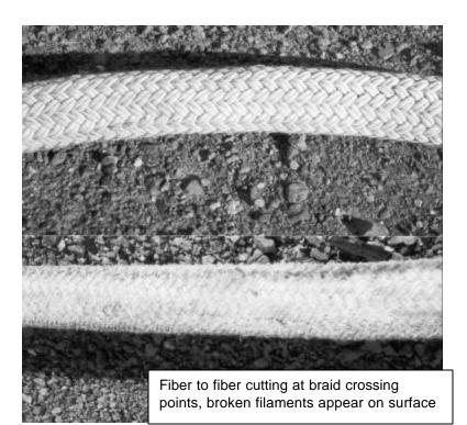
Figure D-001 Fiber Abrasion – Cyclic Tension Undamaged - Upper Photo
