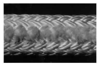
Figure D-007 Localized External Abrasion
